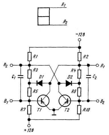
Fig. 10 - Schematic circuit diagram and logic symbol of a flip-flop.
