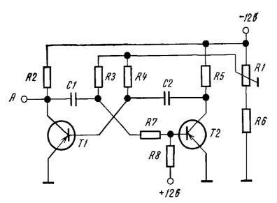
Fig. 9 - Schematic circuit diagram and logic symbol of a multivibrator.
