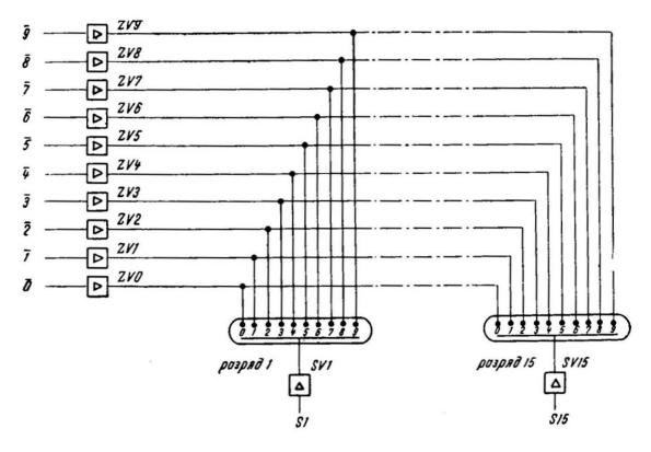
Fig. 31. Circuit diagram for connecting cathode amplifiers to the numerical cathodes of the display.
