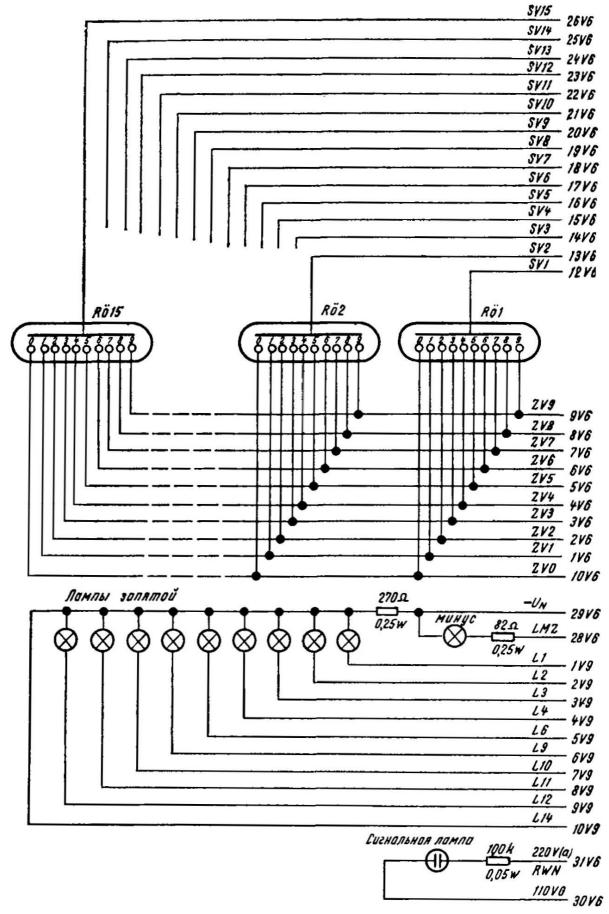
Fig. 26. Schematic Circuit diagram of the display unit.
