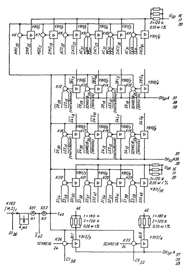
Fig. 35. Functional diagram of board 2.
