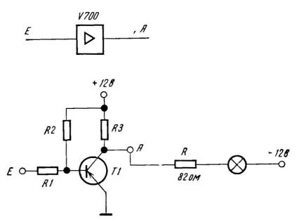
Fig. 12 - Schematic circuit diagram and logic symbol of the "minus" indicator lamp.
