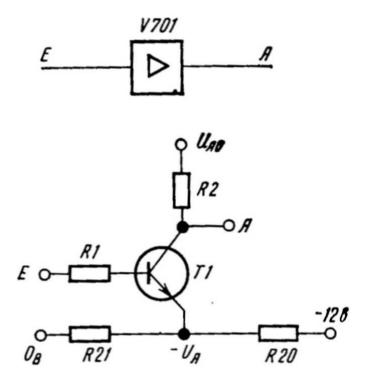
Fig. 13. Schematic circuit diagram and logic symbol of the display cathode driver.
