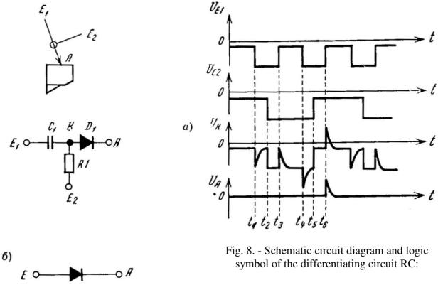
Diode D1 - 1N35 or GAZ17; Capacitor C1 - 560pF 5% 63V; Resistor R1-10k 0,05 W 10%; A) - diagram of the formation of signals by the differentiating circuit with a control input; B) the diode of the collector input of the flip-flop of 1N35 or GAZ17.
