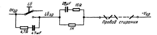
Fig. 27. Schematic circuit diagram of operational register erasure.
