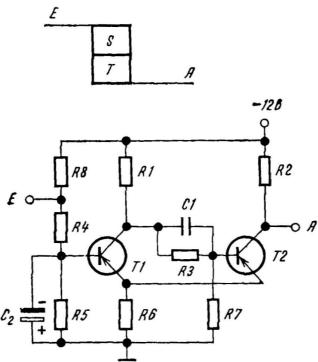
Fig. 16. Schematic circuit diagram of the Schmitt trigger.
