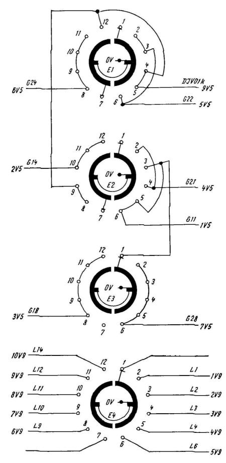
Fig. 22. Circuit diagram of the Decimal Point position switch.
