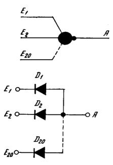
Fig. 4. Logic symbol and circuit diagram of an « OR » gate.
