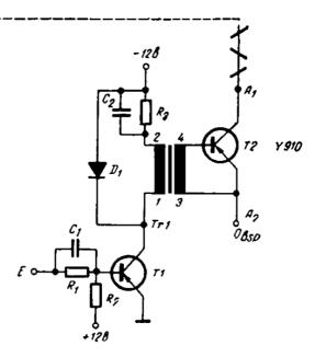
Fig. 17. Schematic circuit diagram and logic diagram of the ferrite core polarity reversal drivers.
