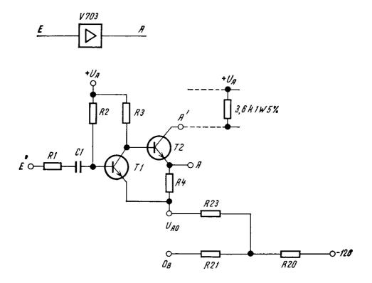
Fig. 14 Schematic circuit diagram and logic symbol of the digital display anode driver.
