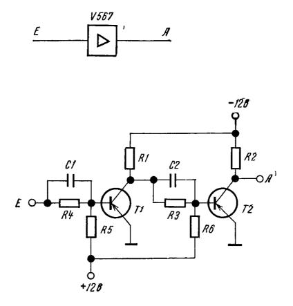
Fig. 6. Logic symbol and circuit diagram of a "Driver amplifier". Component parts of V567
