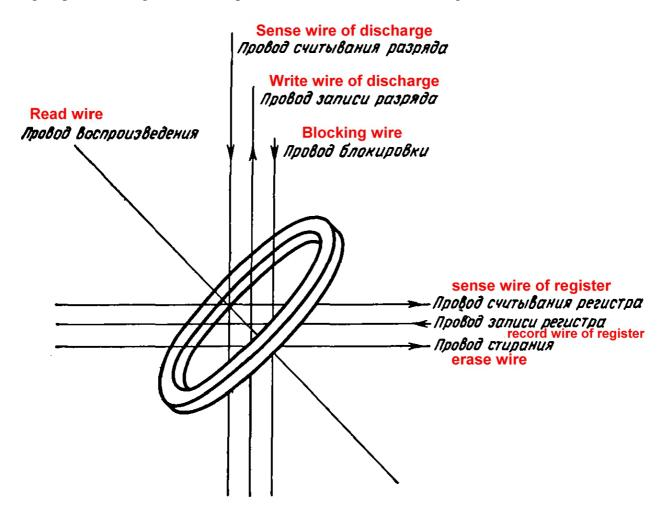
Fig. 24. Diagrammatic representation of a ferrite core.
