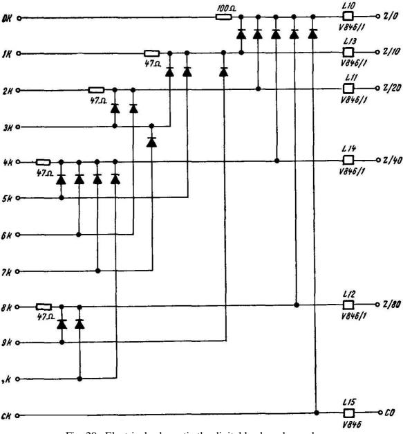
Fig. 20, Electrical schematic the digital keyboard encoder.
