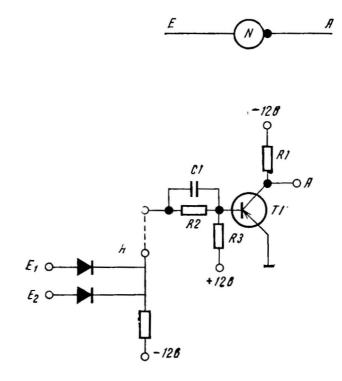
Fig 5. Logic symbol, and circuit diagram of an "Inverter". Component parts:
