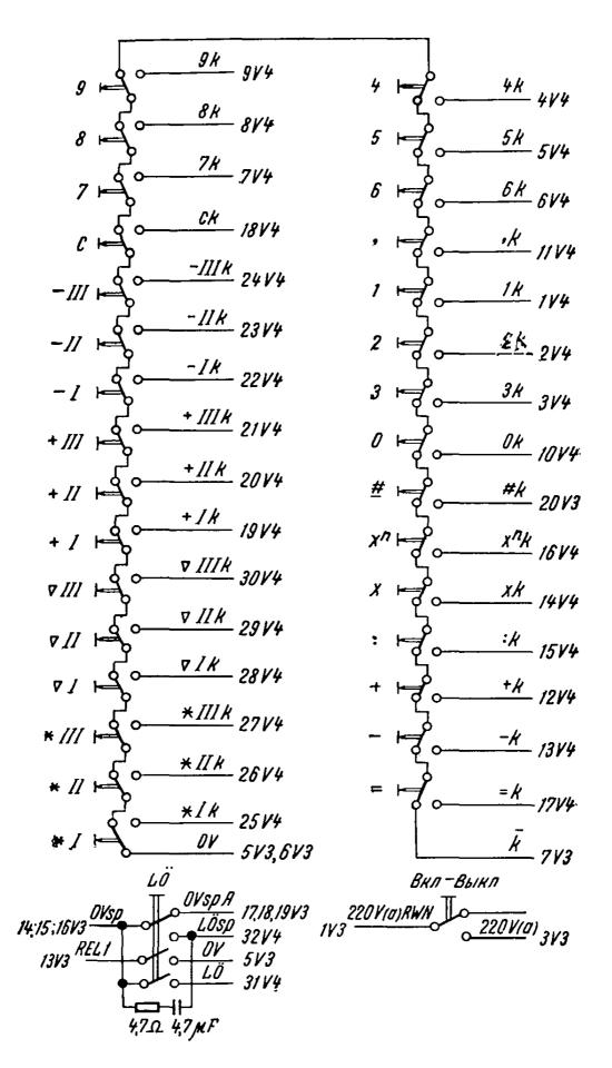
Fig. 19. Keyboard Input unit circuit diagram.
