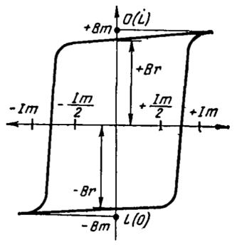
Fig. 23. Ferrite core hysteresis loop.
